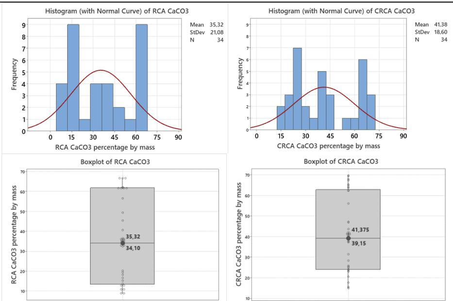
Fig. 5  $\text{CaCO}_3$  content per mass (%) statistical variables for RCA and CRCA
