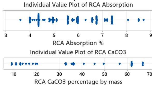
Fig. 2 Absorption distribution and CaCO<sub>3</sub> content of the RCA form the data base
