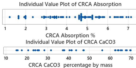
Fig. 3 Absorption distribution and  $\text{CaCO}_3$  content of the CRCA from the data base
