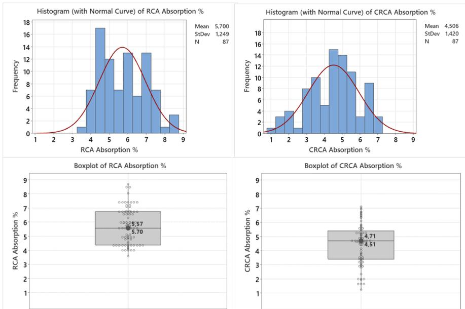
Fig. 4 Water absorption (w) statistical variables for RCA and CRCA
