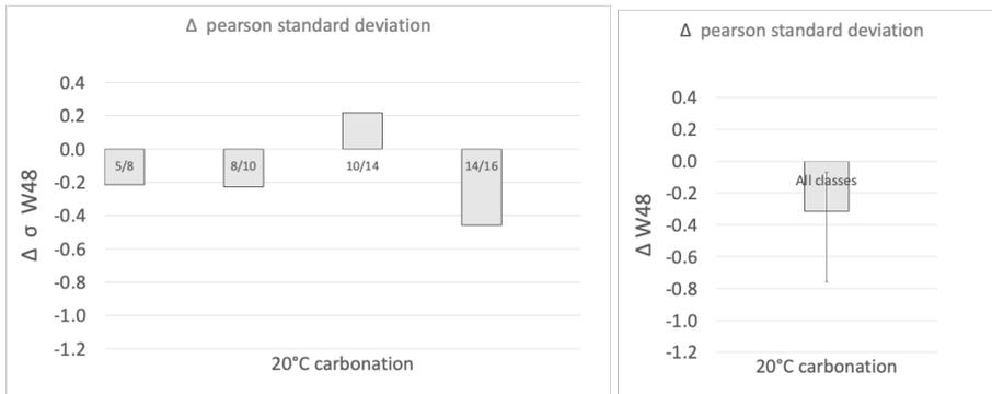
Fig. 11 RCA and CRAC water absorption variability for 20°C carbonation
