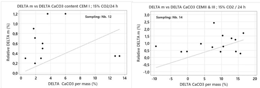
Fig. 8 Comparisons of RCA to CRCA properties variations - 15% CO<sub>2</sub> for 24h.
