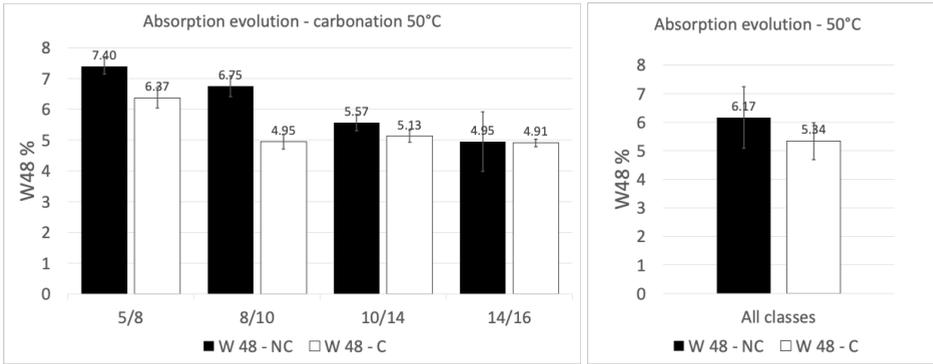
Fig. 10 RCA and CRAC water absorption for 50°C carbonation
