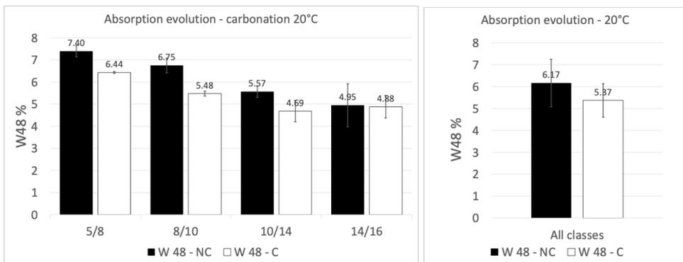
Fig. 9 RCA and CRAC water absorption for 20°C carbonation
