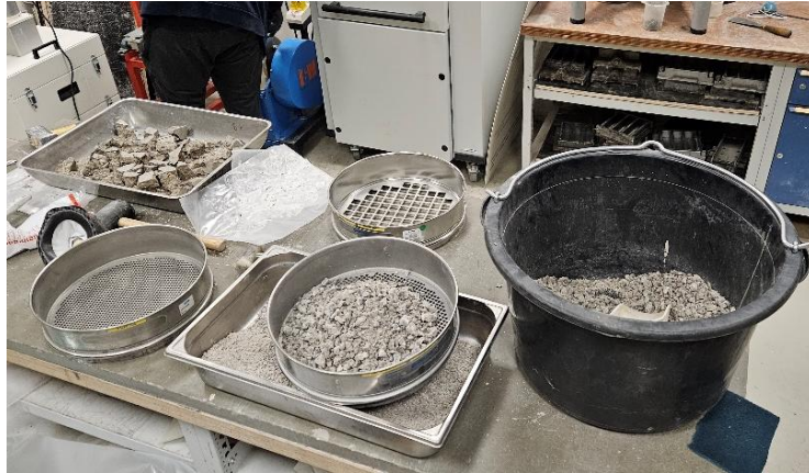
Fig. 1 Sieving process in laboratory of the concrete aggregates
