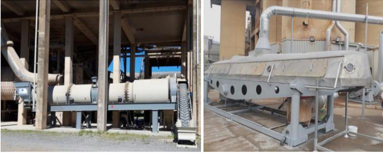
Fig. 3 Two demonstrators developed during the project FastCarb. Left: rolling drum reactor at the Créchy plant (©Vicat). Right: fluidized bed reactor at the Val d'Azergues plant (©Holcim).
