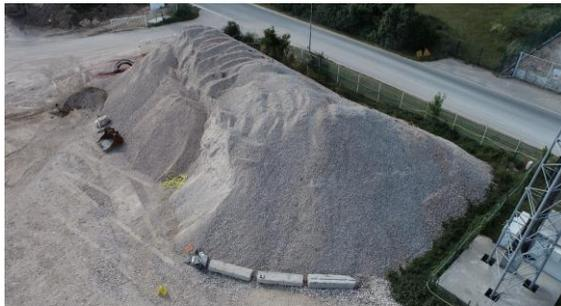
Fig. 1 Studied stockpile of RCA in La Rochelle (France) photographed by drone.
